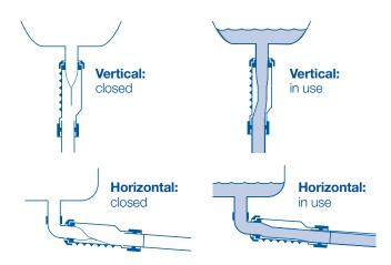
The  ${\sf Hep_VO}$  Sanitary Waste Valve opens under the water pressure of a fixture emptying and closes to form a tight seal after the fixture has discharged.
