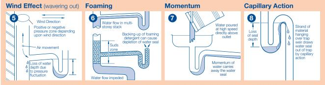
Wind Effect: air movement across the top of the Soil & Vent Pipe causes reciprocation of water in the trap and potential for loss of seal depth. Foaming: agitation of waste water containing detergents in the Soil and Vent pipe creates foaming which pushes water out of the trap.
